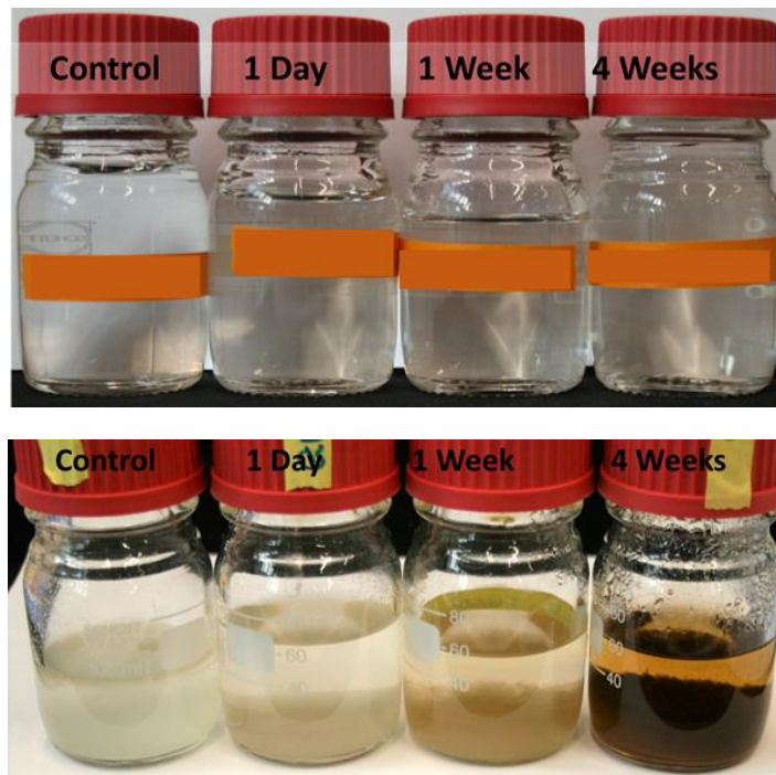
Example of thermally stable (top) and thermally unstable (bottom) DRA under geothermal and district heating conditions
